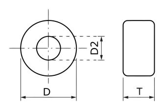
General Information Series ESD-R Style Round - Toroidal Cable Type Round Cable EMI Core Solid, For Round Cables, Toroidal Cores, Description Bare Type RoHS Yes UL94 V-2 Qualifications Materials Mn-Zn
