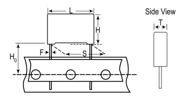
**General Information** Series R46 275 VAC Dielectric Metallized Polypropylene Style Radial Features **EMI** Safety RoHS Yes Lead Wire Leads Safety Class X2 ENEC, UL, cUL, CQC Qualifications AEC-Q200 No **THB** Performance No **Component Weight** 1.698 g We Recommended To Use R46 @ 310 VAC. Notes
