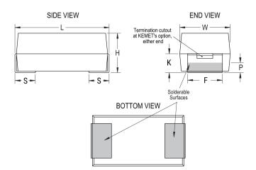
Series T419 CWR19 MnO2 Tantalum Dielectric Style SMD Chip Description SMD, MnO2, Molded, Military Equivalent RoHS No 🛕 WARNING: Cancer and reproductive harm -Prop 65 http://www.p65warnings.ca.gov. SCIP Number 1dd2e1b8-26dd-4d52-927c-6f9d519011aa Termination Solder Coated Qualifications MIL-PRF-55365/11, CWR19 Style AEC-Q200 No Component 68.73 mg Weight Note: When Option C Is Selected For Lead Notes Material, Add An Additional 0.38mm To The Tolerances For "L", "W", "H", "K", "F" And "S". MSL 1
