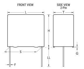
**General Information** Series PFR/F411 Dielectric Film/Foil Polypropylene Style Radial Features Pulse RoHS Yes Lead Wire Leads AEC-Q200 No Component 0.36 g Weight An Operating Temperature Up To +105C Is Allowed Under Certain Conditions. Please Consult Miscellaneous KEMET For Details.
