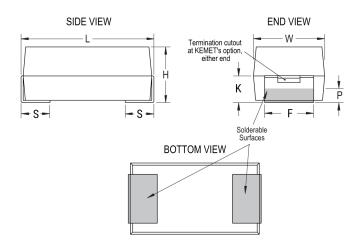
**General Information** Series T429 CWR29 MnO2 Tantalum Dielectric Style SMD Chip Description SMD, MnO2, Molded, Military Equivalent, Low ESR RoHS Yes Termination Gold Qualifications MIL-PRF-55365/11, CWR29 Style AEC-Q200 No Component 173.63 mg Weight Note: When Option C Is Selected For Lead Notes Material, Add An Additional 0.38mm To The Tolerances For "L", "W", "H", "K", "F" And "S". MSL 1
