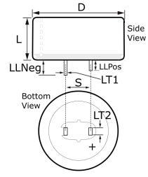
General InformationSeriesFGHDescriptionRadial Cylindrical Double Layer CapacitorRoHSYesAEC-Q200NoComponent Weight1.3 gMiscellaneousDischargeValue = 0.22 F.
