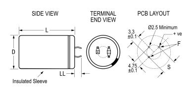
**General Information** Series ALA8A Dielectric Aluminum Electrolytic Description Snap-In, Aluminum Electrolytic RoHS Lead 3 Pin Short Qualifications AEC-Q200 AEC-Q200 Yes Halogen Free Yes Component Weight 75 g Shelf Life 156 Weeks
