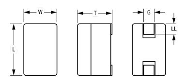
**General Information** Series TPI Style SMD Chip Size 078060(4431) Description Surface Mount Inductor Features AC Optimized TPI Inductors **RoHS** Yes Core Ferrite 40 (K) Temperature Rise Max. Miscellaneous
