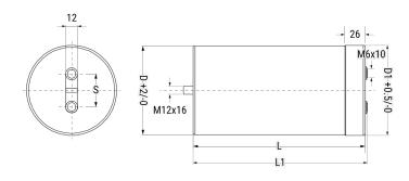
General Information Series C44U-M Dielectric Metallized Polypropylene Style Features DC Filtering, Energy Storage RoHS With Exemptions **REACH** SVHC (Pb - CAS 7439-92-1) SCIP Number cc1c1ec4-db9e-4815-b26b-e8a34ddfb776 Screw Terminals M6 Lead AEC-Q200 No Component 1320 g Weight Thermal Resistance = 3.8 C/W. Weight = 6600 Miscellaneous grams.
