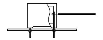
Temperature monitored inside the capacitor.
