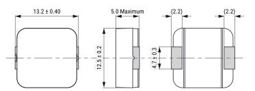
**General Information** Series MPX Style SMD Chip Size 1250(5350) Description Surface Mount Inductor Features Power Inductors **RoHS** Yes Core Composite Miscellaneous 40 (K) Temperature Rise Max.
