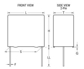
**General Information** Series F611 Dielectric Metallized Polyester Style Radial MKT (Wound), DC Multipurpose Applications Features RoHS Yes Lead Wire Leads AEC-Q200 No Component 28.5 g Weight The Rated Voltage Decreases 1.25%/C Between +85C And +105C (For +125C, Please Consult Kemet). ClimCat: 55/105/56. Miscellaneous
