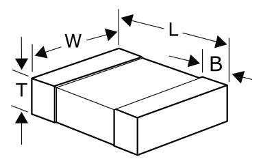
Series VE Type Varistors Style SMD Chip Description Surface Mount Varistors Features Low Voltage High Temperature Termination Nickel Tin RoHS Yes Qualifications IEC, UL, AEC-Q200 AEC-Q200 Yes
