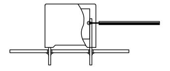
Temperature monitored inside the capacitor.
