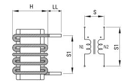
General InformationSeriesSCFStyleThrough-HoleRoHSYesNotesLead Spacing (S/S1) Are For Reference Only.MiscellaneousTemperature Rise Maximum: 55 KCoreNanocrystal
