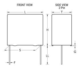
**General Information** Series F461 Dielectric Metallized Polypropylene Style Radial MKP, Pulse Features RoHS Yes Lead Wire Leads AEC-Q200 No Component 1.213 g Weight The Rated Voltage Decreases 2%/C Between +85C And +105C (1.25%/C For AC). ClimCat: Miscellaneous 55/105/56.
