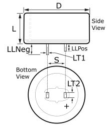
General InformationSeriesFSDescriptionRadial Cylindrical Double Layer CapacitorRoHSYesAEC-Q200NoComponent Weight1.6 gMiscellaneousDischargeValue = 0.033 F.
