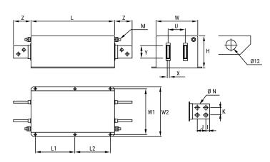
**General Information** Series FLLE2-PV Style Chassis Mount Description EMI Filter, With Y Capacitor Single Phase, Photovoltaic Applications Features Phase Single-phase RoHS Yes Qualifications IEC/EN 60939, UL 1283 Threaded Studs M16 **Terminal Type**
