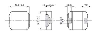
**General Information** Series MPXV Style SMD Chip Size 1040(4340) Description Surface Mount Inductor Features Power Inductors RoHS Yes Qualifications AEC-Q200 AEC-Q200 Yes Core Composite 40 (K) Temperature Rise Max. Miscellaneous
