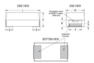
Series T419 CWR19 MnO2 Tantalum Dielectric Style SMD Chip Description SMD, MnO2, Molded, Military Equivalent RoHS No 🛕 WARNING: Cancer and reproductive harm – Prop 65 http://www.p65warnings.ca.gov. SCIP Number 1dd2e1b8-26dd-4d52-927c-6f9d519011aa Termination Solder Coated Qualifications MIL-PRF-55365/11, CWR19 Style AEC-Q200 No Component 421.63 mg Weight Note: When Option C Is Selected For Lead Notes Material, Add An Additional 0.38mm To The Tolerances For "L", "W", "H", "K", "F" And "S". MSL 1
