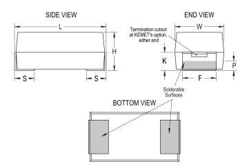
Style SMD Chip Description SMD, MnO2, Molded, Military Equivalent RoHS No 🛕 WARNING: Cancer and reproductive harm – Prop 65 http://www.p65warnings.ca.gov. SCIP Number 656db0b8-8445-4117-82f2-2f12e764f0b1 Termination Solder Fused Qualifications MIL-PRF-55365/4, CWR09 Style AEC-Q200 No Component 266.42 mg Weight Note: When Option C Is Selected For Lead Notes Material, Add An Additional 0.38mm To The Tolerances For "L", "W", "H", "K", "F" And "S". MSL 1
