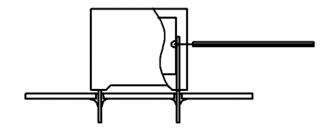
Temperature monitored inside the capacitor.
