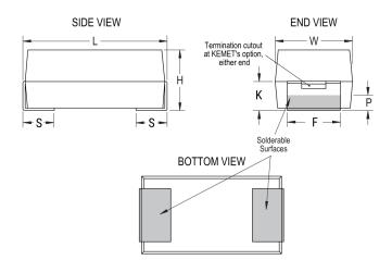
MnO2 Tantalum Dielectric Style SMD Chip Description SMD, MnO2, Molded, Military Equivalent RoHS No 🛕 WARNING: Cancer and reproductive harm – Prop 65 http://www.p65warnings.ca.gov. SCIP Number 652b281f-d242-4453-bc44-0655d646cec3 Termination Hot Solder Dipped Qualifications MIL-PRF-55365/11, CWR19 Style AEC-Q200 No Component 173.63 mg Weight Note: When Option C Is Selected For Lead Notes Material, Add An Additional 0.38mm To The Tolerances For "L", "W", "H", "K", "F" And "S". MSL 1
