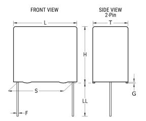
**General Information** Series F611 Dielectric Metallized Polyester Style Radial MKT (Wound), DC Multipurpose Applications Features RoHS Yes Lead Wire Leads AEC-Q200 No Component 14 g Weight The Rated Voltage Decreases 1.25%/C Between +85C And +105C (For +125C, Please Consult Kemet). ClimCat: 55/105/56. Miscellaneous
