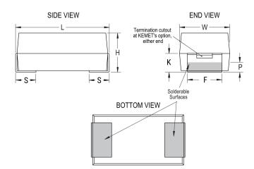
**General Information** Series T497 HRA Dielectric MnO2 Tantalum Style SMD Chip Description SMD, MnO2, Molded, High Reliability, Medical Features High Reliability, Medical RoHS Yes Termination Tin Qualifications CWR09/19/29 Style AEC-Q200 No Component 68.73 mg Weight Note: When solder coated terminations are Notes required, add an additional 0.38mm (0.015inch) to the tolerances for "L", "W", "H", "K", "F" and "S". MSL 1
