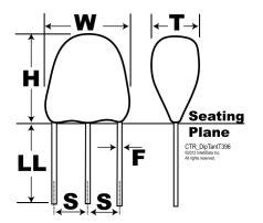
Series T396 Dielectric MnO2 Tantalum Style **Radial Three Lead** Description Radial, Solid Tantalum, Three Leaded RoHS No 🛕 WARNING: Cancer and reproductive harm – Prop 65 http://www.p65warnings.ca.gov. SCIP 78c25989-fc86-4b0d-a598-1bcecbae95c0 Number Termination Lead (SnPb) AEC-Q200 No Construction Conformal Notes Longest Lead Is Positive.
