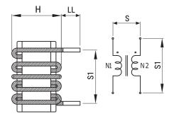
General InformationSeriesSC-DStyleThrough-HoleRoHSYesNotesLead Spacing (S/S1) Are For Reference Only.MiscellaneousTemperature Rise Maximum: 50 KCoreNi-Zn Ferrite
