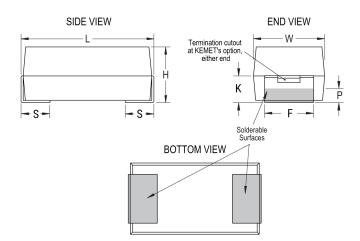
**General Information** Series T409 CWR09 MnO2 Tantalum Dielectric Style SMD Chip Description SMD, MnO2, Molded, Military Equivalent RoHS Yes Termination Gold Qualifications MIL-PRF-55365/4, CWR09 Style AEC-Q200 No Component 349.01 mg Weight Note: When Option C Is Selected For Lead Notes Material, Add An Additional 0.38mm To The Tolerances For "L", "W", "H", "K", "F" And "S". MSL 1
