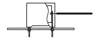
Temperature monitored inside the capacitor.
