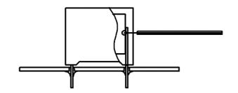
The temperature is monitored inside the capacitor.
