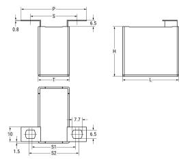
**General Information** Series C4BS Dielectric Metallized Polypropylene Style Radial IGBT Circuit Features RoHS Yes Lead Flat Tabs AEC-Q200 No **Component Weight** 53.5 g Miscellaneous KEMET Style T Tabs.
