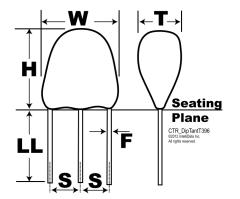
Series T396 Dielectric MnO2 Tantalum Style **Radial Three Lead** Description Radial, Solid Tantalum, Three Leaded RoHS Yes Termination Tin AEC-Q200 No Construction Conformal Notes Longest Lead Is Positive.
