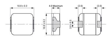
**General Information** Series MPXV Style SMD Chip Size 1040(4340) Description Surface Mount Inductor Features Power Inductors RoHS Yes Qualifications AEC-Q200 AEC-Q200 Yes Core Composite 40 (K) Temperature Rise Max. Miscellaneous
