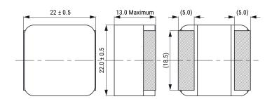
**General Information** Series MPX Style SMD Chip Size 2213(9088) Description Surface Mount Inductor Features Power Inductors **RoHS** Yes Core Composite Miscellaneous 40 (K) Temperature Rise Max.
