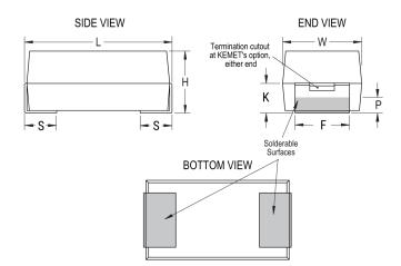
MnO2 Tantalum Dielectric Style SMD Chip Description SMD, MnO2, Molded, Military Equivalent RoHS No MARNING: Cancer and reproductive harm -Prop 65 http://www.p65warnings.ca.gov. Termination Hot Solder Dipped Qualifications MIL-PRF-55365/11, CWR19 Style AEC-Q200 No Component 349.01 mg Weight Note: When Option C Is Selected For Lead Material, Notes Add An Additional 0.38mm To The Tolerances For "L", "W", "H", "K", "F" And "S". MSL 1
