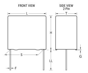
**General Information** Series F462 Dielectric Metallized Polypropylene Style Radial MKP, Pulse Features RoHS Yes Lead Wire Leads AEC-Q200 No Component 0.798 g Weight The Rated Voltage Decreases 2%/C Between +85C And +105C (1.25%/C For AC). ClimCat: Miscellaneous 55/105/56.
