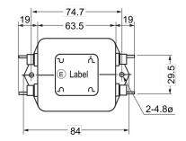
**General Information** Series GT Style Metal Box Description Noise Filters RoHS With Exemptions Qualifications UL, CSA, TUV Miscellaneous 35 K Self-Temperature Rise Max. Lead Fast On Terminal Type Faston
