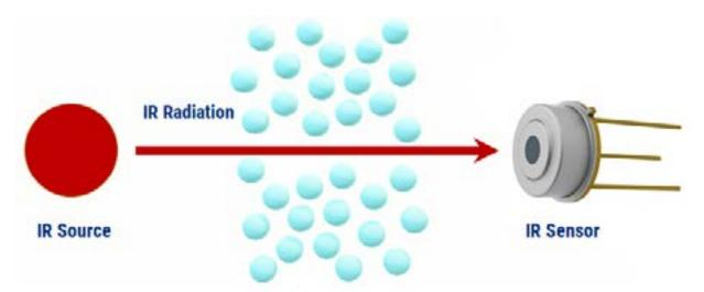
The IR source is directed as energy towards the sensor like an IR spotlight. Depending on the specific gas of interest or gas concentration levels between the IR source and the pyroelectric sensor, the IR transmitted is absorbed by the presence of the gas by a small amount. Understanding how much IR is being optically transmitted versus how much is received can indicate gas concentration levels.
