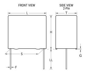
Series PHE450/F450 Dielectric Double Metallized Polypropylene Style Radial Features Pulse RoHS Yes Lead Wire Leads AEC-Q200 No Component 9 g Weight The Rated Voltage Decreases 1.3%/C Between Miscellaneous +85C And +105C. Rthha= 34 C/W (85C), 0.2 m/s.
