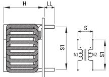
**General Information** Series SC-JH Style Through-Hole RoHS Yes Lead Spacing (S/S1) Are For Reference Only. Notes Miscellaneous Temperature Rise Maximum: 50 K Core Mn-Zn Ferrite
