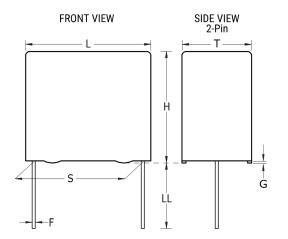
**General Information** Series F462 Dielectric Metallized Polypropylene Style Radial MKP, Pulse Features RoHS Yes Lead Wire Leads AEC-Q200 No Component 28.5 g Weight The Rated Voltage Decreases 2%/C Between +85C And +105C (1.25%/C For AC). ClimCat: Miscellaneous 55/105/56.
