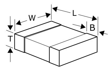
Туре Varistors Style SMD Chip Description Surface Mount Varistors Features Low Voltage High Temperature Termination Nickel Tin RoHS Yes Qualifications IEC, UL, AEC-Q200 AEC-Q200 Yes
