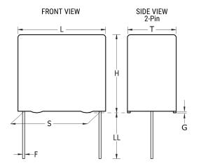
**General Information** Series PFR/F411 Dielectric Film/Foil Polypropylene Style Radial Features Pulse RoHS Yes Lead Wire Leads AEC-Q200 No Component 0.386 g Weight An Operating Temperature Up To +105C Is Allowed Under Certain Conditions. Please Consult Miscellaneous KEMET For Details.
