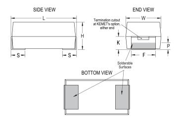
Series T497 HRA Dielectric MnO2 Tantalum Style SMD Chip Description SMD, MnO2, Molded, High Reliability, Medical Features High Reliability, Medical RoHS Yes Termination Tin Qualifications CWR09/19/29 Style AEC-Q200 No Component 173.63 mg Weight Note: When solder coated terminations are Notes required, add an additional 0.38mm (0.015inch) to the tolerances for "L", "W", "H", "K", "F" and "S". MSL
