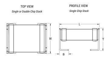
General Information Series KPS SMD Comm X7R Style Stacked Chip SMD, MLCC, Stacked, Single Chip, Temperature Description Stable Features Temperature Stable RoHS Yes Termination Tin AEC-Q200 No Component 170 mg Weight 1812-1 Chip Size Shelf Life 78 Weeks MSL 1
