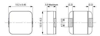
**General Information** Series MPXV Style SMD Chip Size 1250(5350) Description Surface Mount Inductor Features Power Inductors RoHS Yes Qualifications AEC-Q200 AEC-Q200 Yes Core Composite 40 (K) Temperature Rise Max. Miscellaneous
