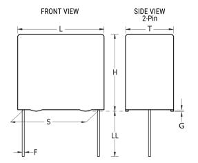
**General Information** Series PFR/F411 Dielectric Film/Foil Polypropylene Style Radial Features Pulse RoHS Yes Lead Wire Leads AEC-Q200 No Component 0.37 g Weight An Operating Temperature Up To +105C Is Miscellaneous Allowed Under Certain Conditions. Please Consult KEMET For Details.
