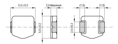
**General Information** Series MPXV Style SMD Chip Size 0520(2120) Description Surface Mount Inductor Features Power Inductors RoHS Yes Qualifications AEC-Q200 AEC-Q200 Yes Core Composite 40 (K) Temperature Rise Max. Miscellaneous
