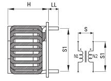
General InformationSeriesSC-JHStyleThrough-HoleRoHSYesNotesLead Spacing (S/S1) Are For Reference Only.MiscellaneousTemperature Rise Maximum: 55 KCoreMn-Zn Ferrite
