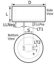
General InformationSeriesFSDescriptionRadial Cylindrical Double Layer CapacitorRoHSYesAEC-Q200NoComponent Weight5.3 gMiscellaneousDischargeValue = 0.33 F.
